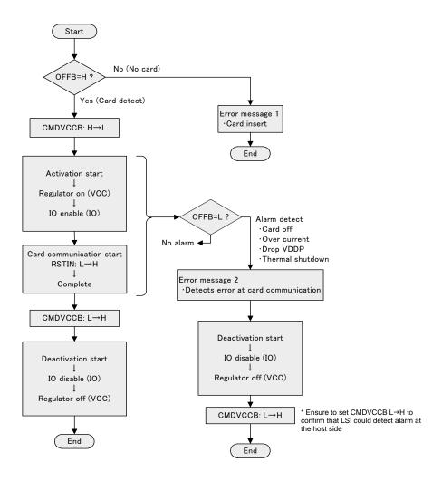
Fig. 7 An example of software control
