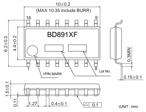
Fig. 3.1 SOP16 Package Dimension
