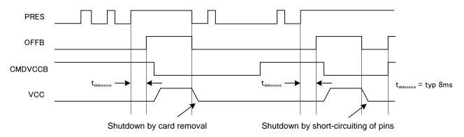
Fig. 6 OFFB, CMDVCCB, PRES, VCC operation
